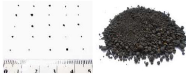
Figure 3. Buton Granular Asphalt (BGA) (dimension in mm).
