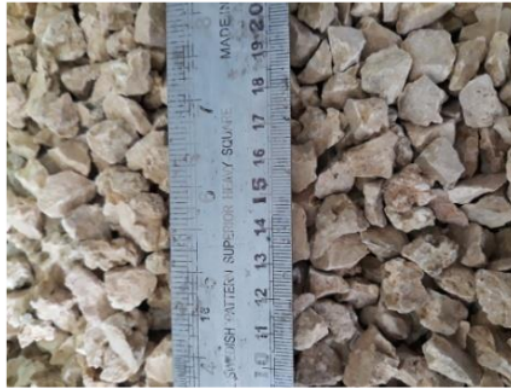
Figure 2. Limestone (dimension in mm).
